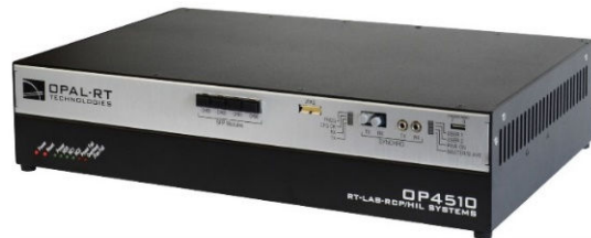
OPAL-RT 4510-4512 / Typhoon HIL: Real-time model of the smart grid/microgrid
