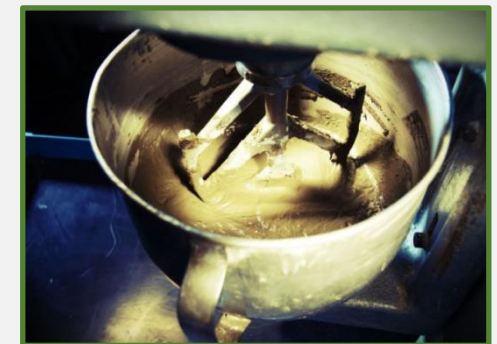
Amasado de Ultra High Performance Concrete
